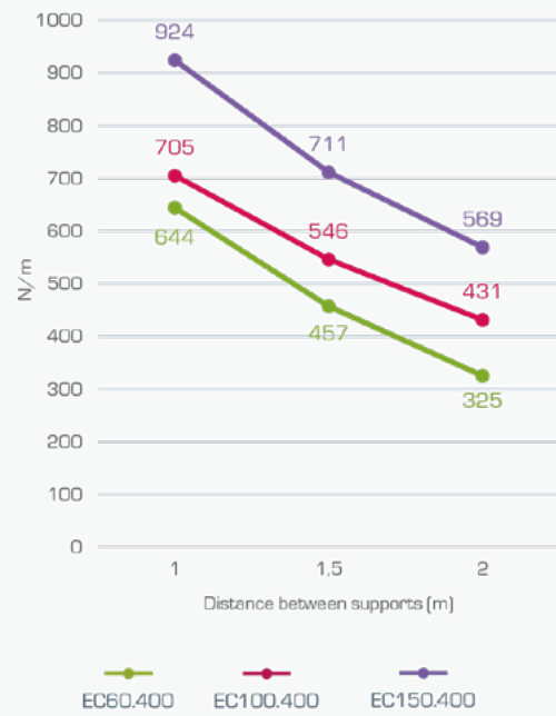
Safe working loads 400mm width basket trays
